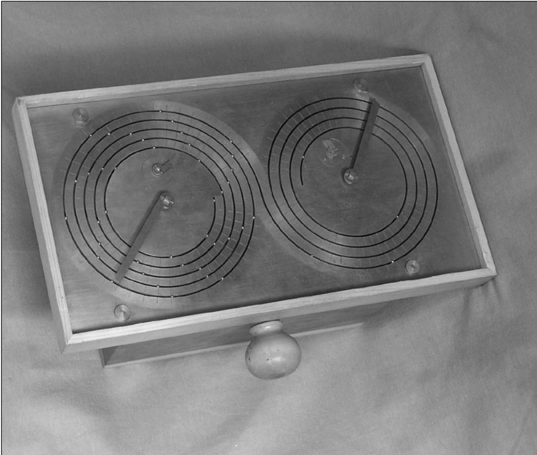
Fig. 6 *The Antikythera Mechanism, reconstruction by M.T.Wright: the back dial.*
