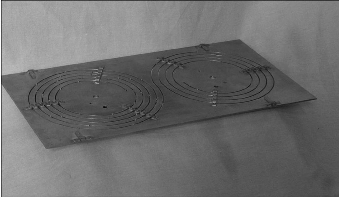
Fig. 7 *The Antikythera Mechanism, reconstruction by M.T.Wright. Back dial plate, inside view.*
